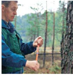
Suunto increment borers are used for examining wood quality and measuring growth rates.
