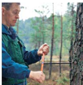
Suunto increment borers are used for examining wood quality and measuring growth rates.
