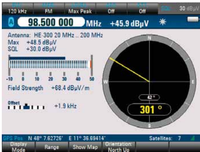
Direction-finding of a signal source with the R&S®HE300 active directional antenna.
