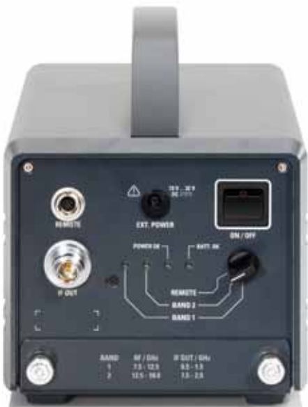
Rear view of the R&S®HF907DC.
