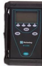
**Model HI-2200 Metering Unit:** This hand-held metering unit contains the processor and readout display for the system's selection of easily connected, interchangeable field probes. The menu driven display has user-selectable readout units and a wide range of field averaging and display options. Up to 65K data points can be logged and uploaded with the built-in RS-232 interface. Four AA alkaline batteries provide a reliable and readily available power source.
