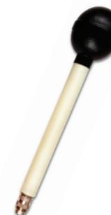
**Model H210 Magnetic Field Probe:** Use this probe to measure magnetic fields across a 300 kHz to 30 MHz frequency range. The H210 is useful for applications such as measurements at AM broadcast installations.
